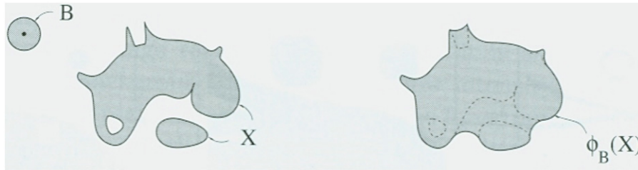
Fig. 1. The effect of a closing operator on a non-smooth object (Reproduced from [42] with permission).
