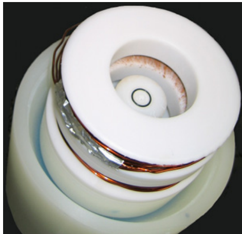
Fig. 1. Experimental configuration of the spin-coater with Helmholtz coils.
