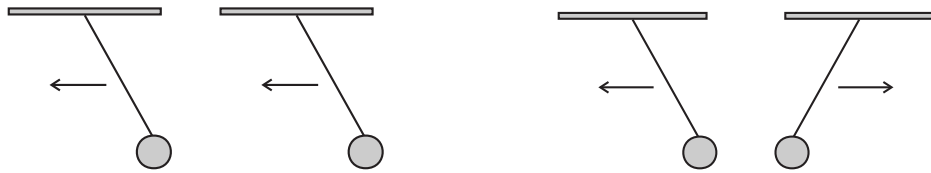
Figure 3: Possible synchronous regimes of two nearly identical oscillators. They may be synchronized in-phase, or in anti-phase.
