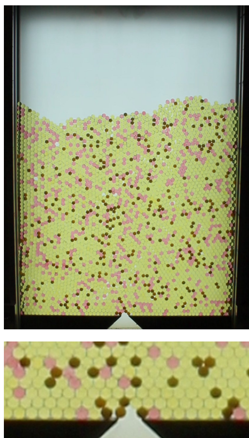
Fig. 1 Top: Image of the container filled with a mixture with 10 % hard frictional beads. Yellow and pink colored hydrogel spheres are equivalent, airsoft bullets appear dark. Bottom: Zoom into the region near the orifice at the bottom, in a clogged state. The orifice in these images is D = 11 mm, slightly less than two particle diameters.
