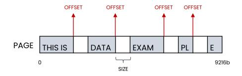
It's necessary to determine the location, size and number of Bad columns within one page of each plane. Location is offset of bad column from the beginning of page. Bad Column size expressed in bytes. Number determines number of offsets from the beginning of page, that must be added in order to cut Bad Column defects.
