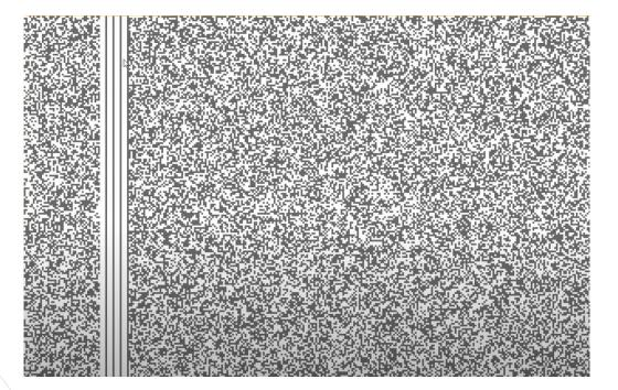
Modern flash controllers employ scrambling algorithms during the data recording process in flash memory. A typical implementation of a scrambler involves the generation of a unique scrambling (XOR) key by the controller, which is then combined with the data through an XOR gate/operation. This occurs for every data block/page before it is written into the flash memory.
